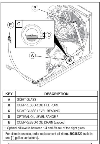
Figure 5-2: Compressor Oil Fill and Oil Charge
