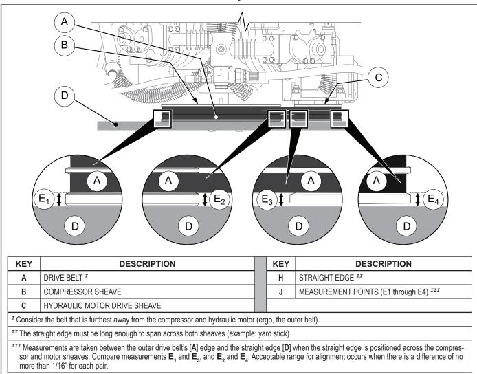
Figure 5-7: Drive Sheave (Pulley) Alignment Check
