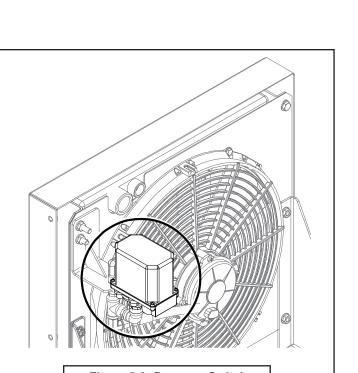
Figure 5-9: Pressure Switch
