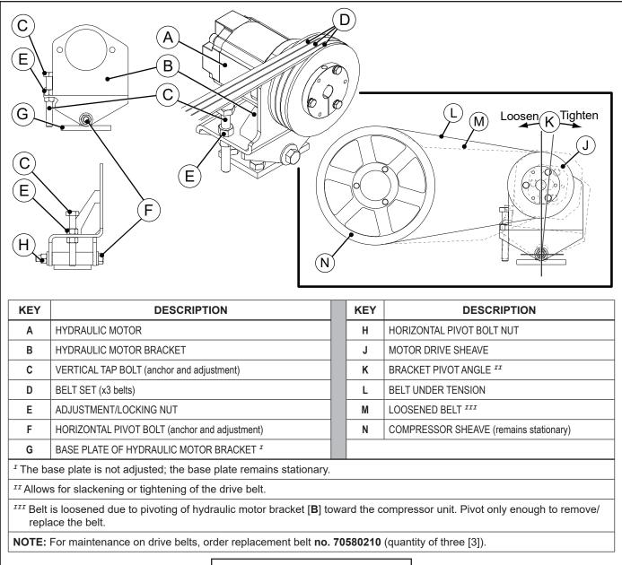
Figure 5-5: Removing Drive Belt
