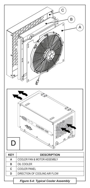
Should the core become clogged, you can use low pressure compressed air to blow through the fins from the inside of the canopy to clean it out. You may need to remove the fan from the shroud in order to reach parts of the core. **DO NOT** use high pressure air or a pressure washer.
