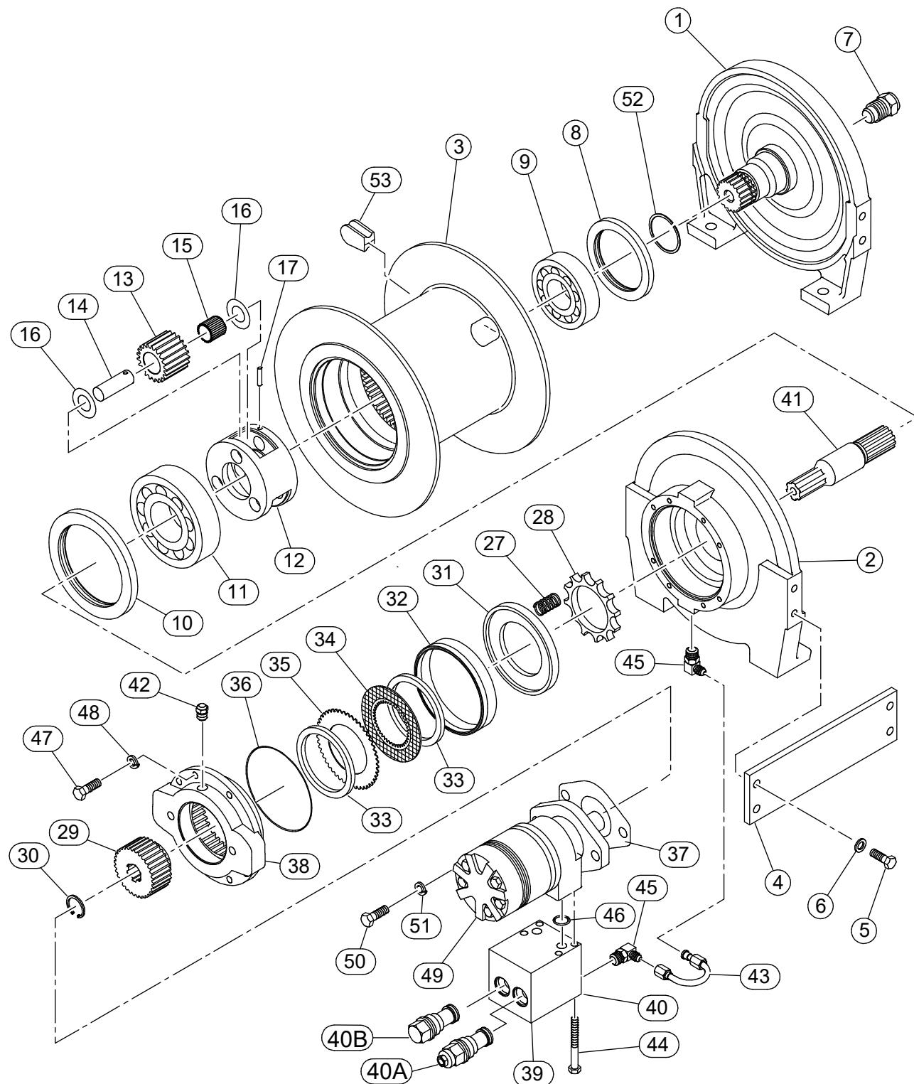
**PLANETARY WINCH (70570761) COMPLETE PARTS LIST**
