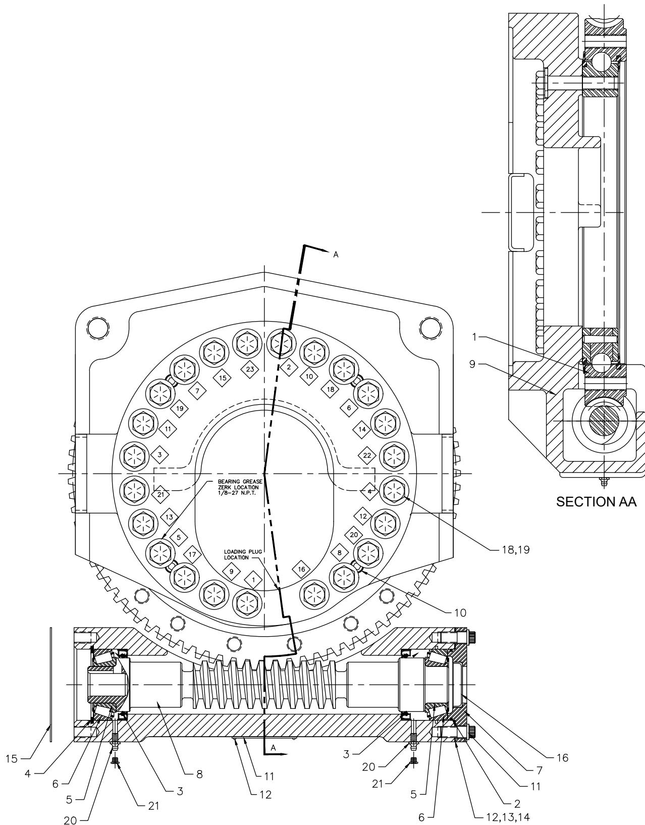
**GEAR ROTATOR (71056543) PARTS LIST**
