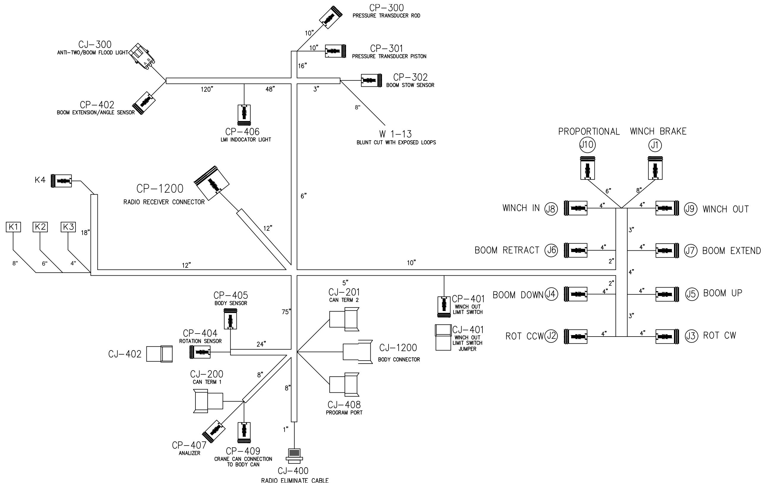
**Harness S4 SP Crane (77441718) Schematic View**
