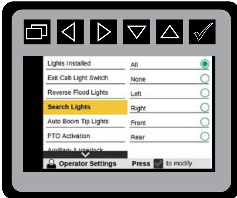
The availability of this function is based on configured set-up found in **Vehicle Configurations**. The **Search Lights** menu will not be shown if the **Search Lights Enabled** is set to NO.
