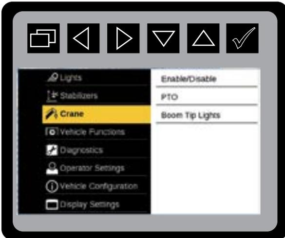
The Crane menu allows the selection of Power On and Power Off options for Crane, PTO, Boom Tip Lights, and Crane Override.
