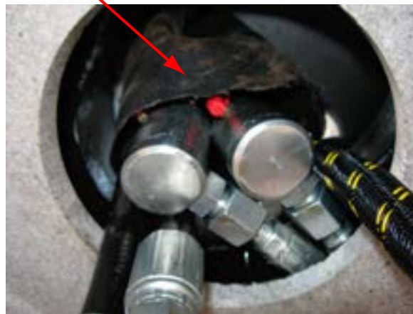
Viewed looking up from crane box. The pressure, return, and rotation hoses are wrapped in the 60350105 hose sleeve.
