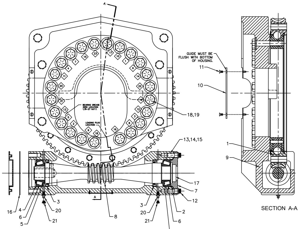
**GEAR ROTATOR (71056577) PARTS LIST**
