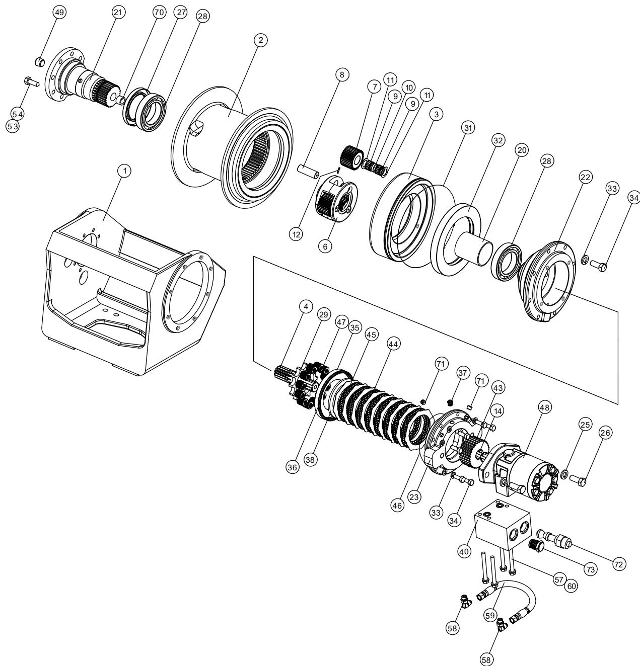
**PLANETARY WINCH (70570771) PARTS LIST**
