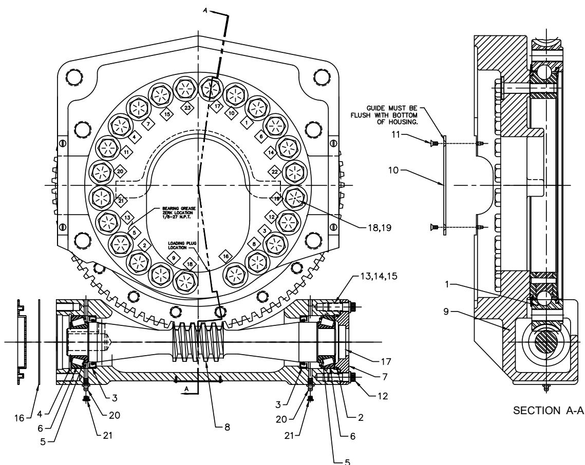
**GEAR ROTATOR (71056577) CONTINUED**
