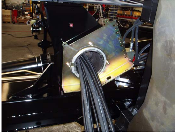
Figure 5 – The underside of the crane with protection plate and hose connection removed.
