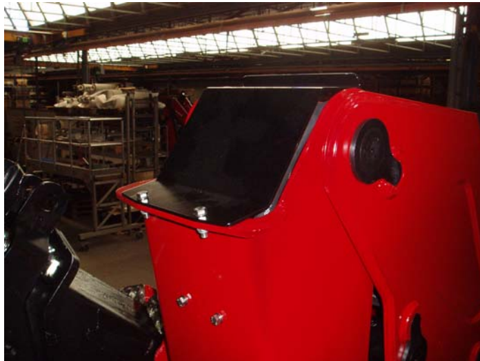
Figure 1 – Photo of the upper part of the column with hose shield
