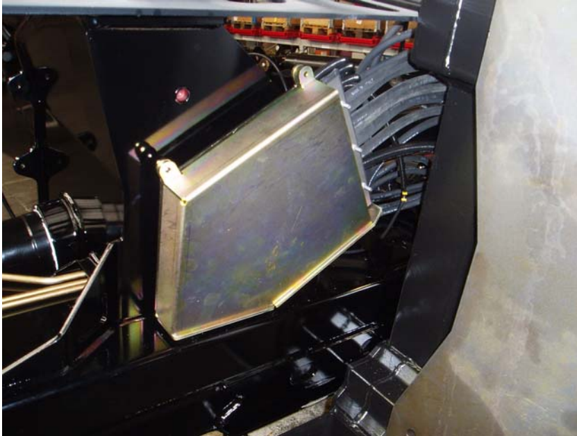
Figure 3 – The underside of the crane with protection plate fitted.
