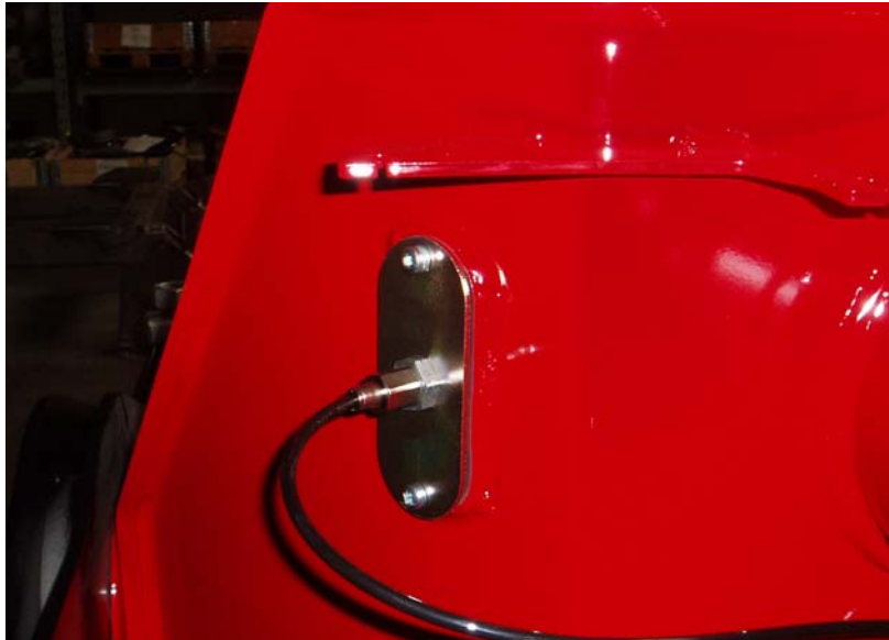
Figure 1 – Cover for lubricating brush on the side of the central part of the base.
