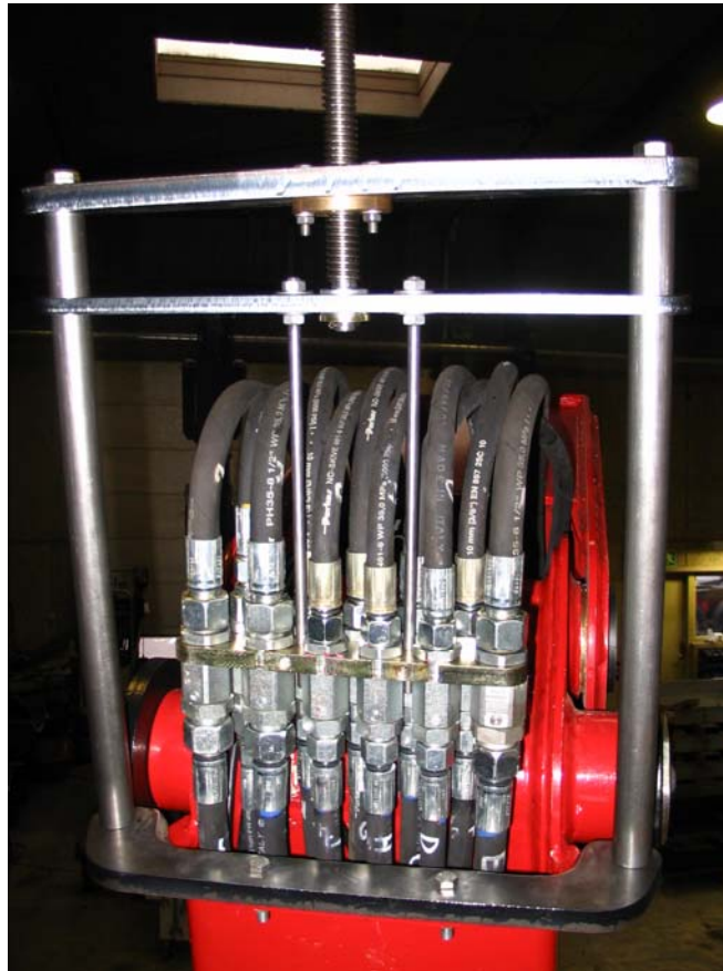
Figure 2 – Photo of the top of the column with the bundle of hoses lifted using the service tools.
