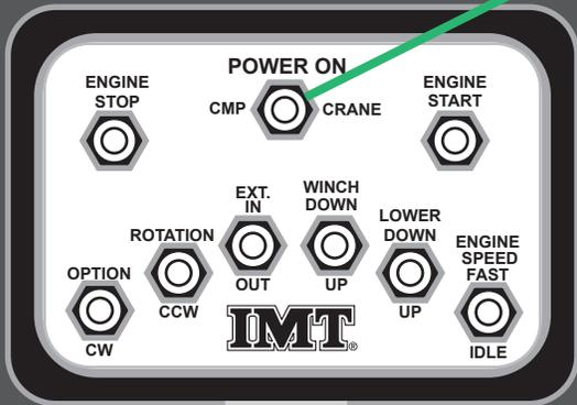
2. On the Tethered Remote Handle Assembly, toggle POWER ON switch (to the right) and back to center 5 times within 5 seconds to start calibration sequence. Leave toggle switch in the OFF (Center) position on the last (5th) sequence.
