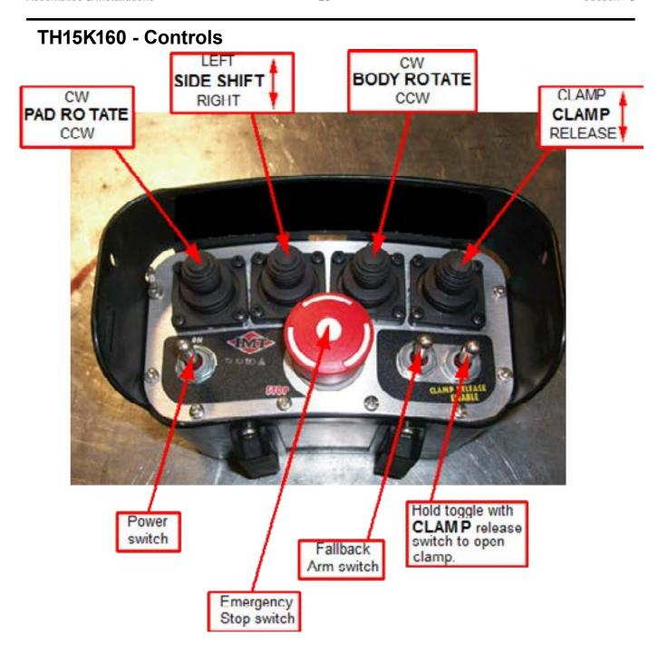
**NOTES:** See the Tirehandler, *Radio Remote System*, IMT manual #99905678, for complete radio remote control system instructions. The Tirehand radio remote control is a cab-mounted or tethered remote with a radio option.
