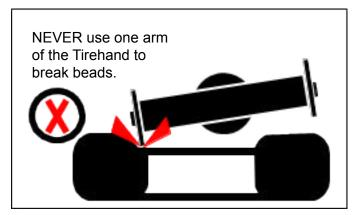
A bead breaker must be used to separate the tire from the rim. It is acceptable to use the Tirehand for holding the sidewall and flange away from the bead while o-rings and locking rings are being installed.
