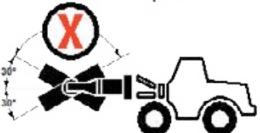
NEVER use the unit for any jacking, pulling or dragging operation involving an object or another vehicle.
