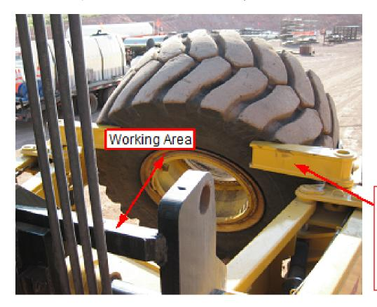
Fallback arms must be deployed when personnel are in the working area between the tire and the carrier vehicle.
