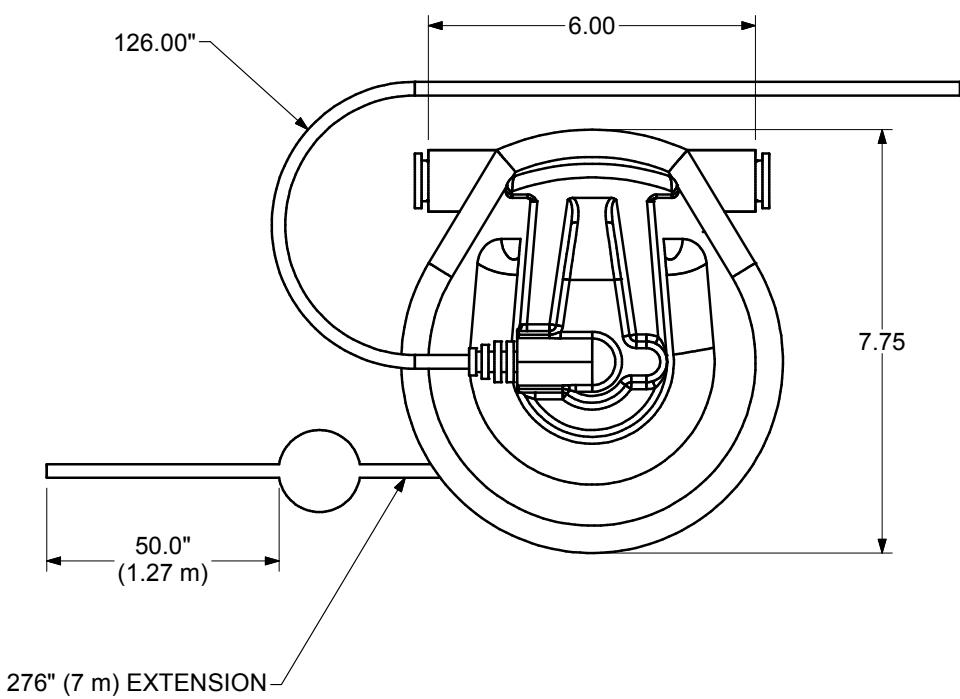
**Cord Reel Assembly, 10'5" W/Packard Connector (51727065)**
