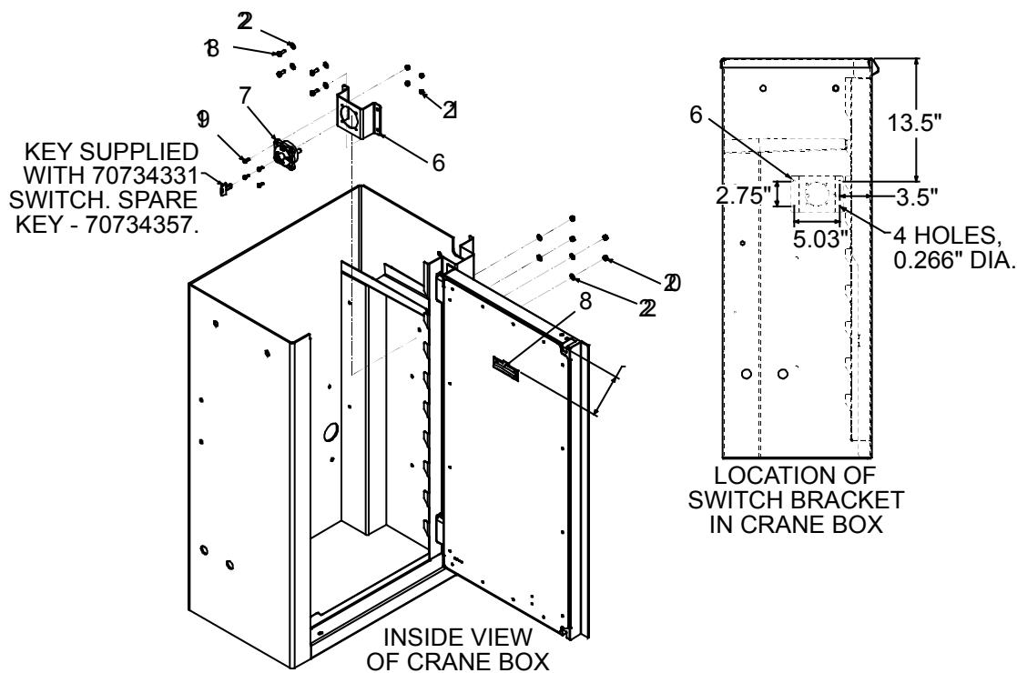
3. Install the vehicle level indicator (item #8) parallel to the door reinforcements.
