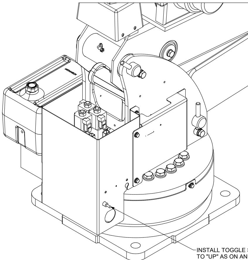
INSTALL TOGGLE SWITCH IN VALVE BANK COVER
