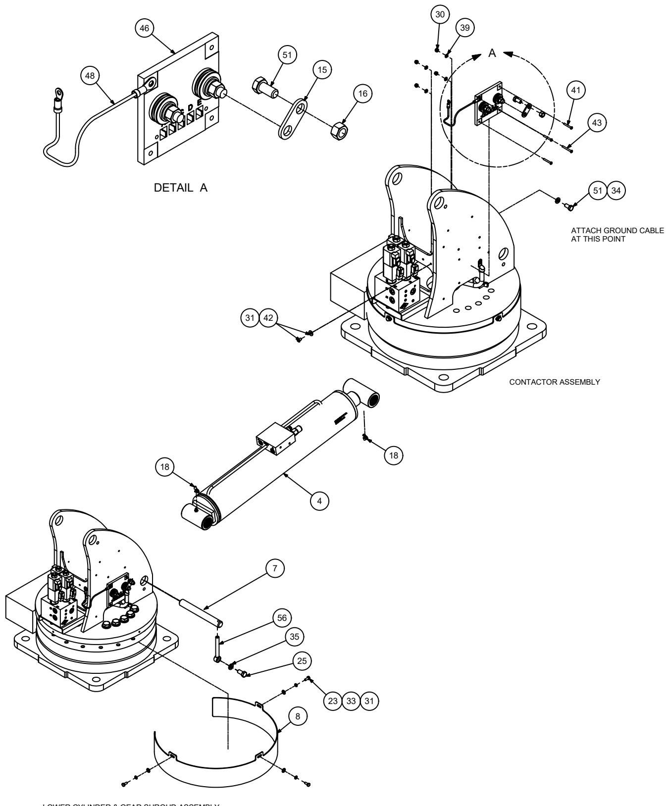
**CONTACTOR ASSEMBLY PARTS LIST (99904454)**
