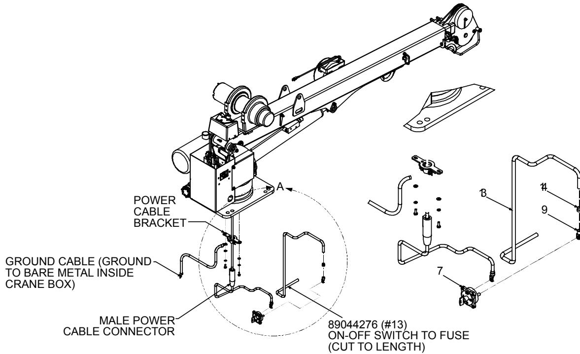
7. Use approximately 4' (1.2 m) of the cable (item #13) to ground both the vehicle battery and auxiliary battery. Connect one end of the ground cable to the negative terminal on the vehicle battery, and the other end to bare metal on the truck body. Use a 5/16" (0.79 cm) ring terminal (item #10 - 77040529) to connect to the truck body.
