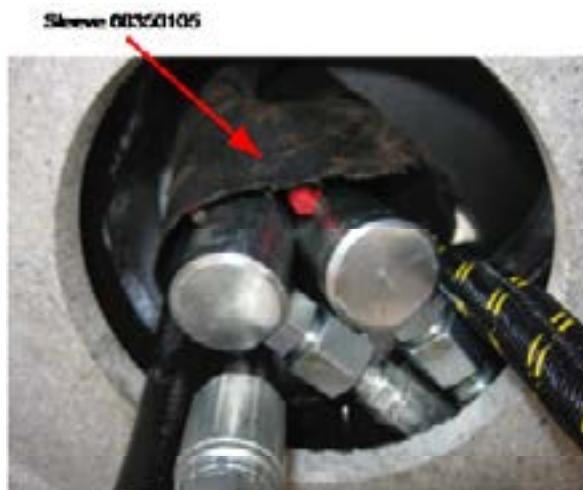
Viewed looking up from crane box. The pressure, return, and rotation hoses are snipped in the 60350105 hose sleeve.
