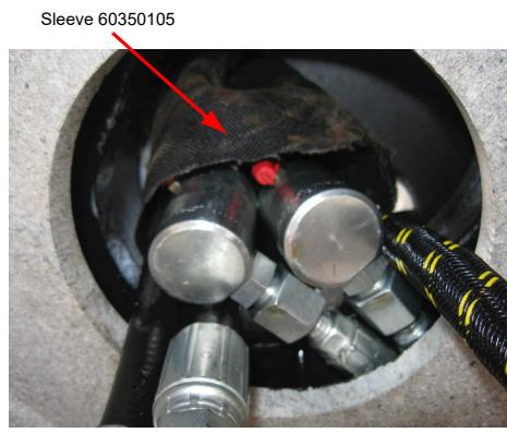
Viewed looking up from crane box. The pressure, return, and rotation hoses are wrapped in the 60350105 hose sleeve.
