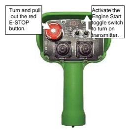
Push and hold the trigger on the inside of the remote handle to use the joystick crane controls.
