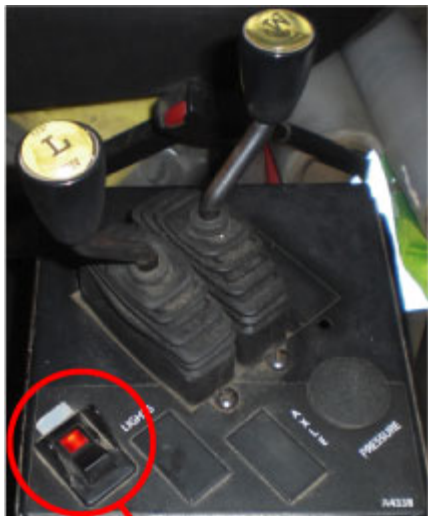
PTO Light ON when PTO is engaged.
