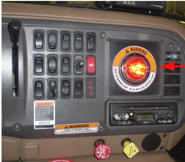
DASH WARNING LIGHT Indicates: Cable Hoist Up Crane Not Stowed Stabilizers Not Stowed
