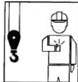
RETRACT BOOM - (Telescoping Booms) - One Hand Signal. One fist in front of chest, thumb pointing outward and heel of fist tapping chest.
