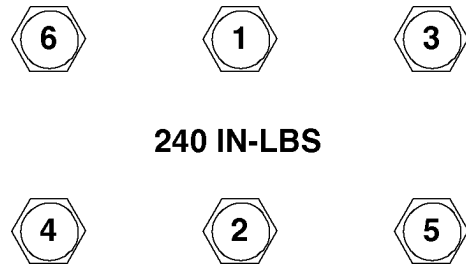
FIGURE E-8. CYLINDER HEAD TORQUE SEQUENCE
