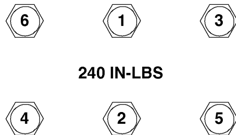
FIGURE E-2. CYLINDER HEAD TORQUE SEQUENCE
