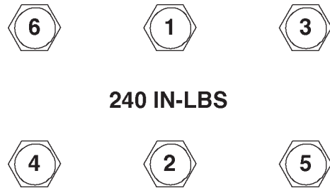
FIGURE E-8. CYLINDER HEAD TORQUE SEQUENCE
