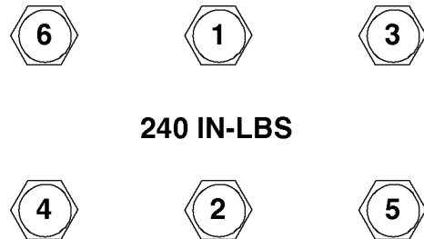
FIGURE E-2. CYLINDER HEAD TORQUE SEQUENCE
