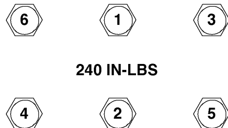
FIGURE E-2. CYLINDER HEAD TORQUE SEQUENCE
