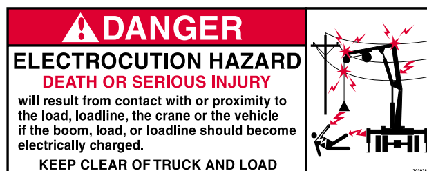
FIGURE G-1. ELECTRICAL HAZARD WARNING DECAL
