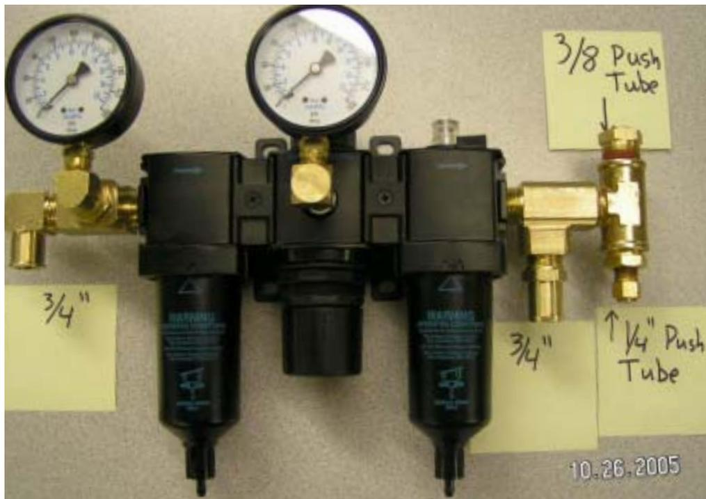
**AIR TANK DRAIN ASSEMBLY (51709358)**
