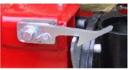
If the loader is equipped with swing-up stabilizer legs they must also be secured in position before driving off. Before the vehicle is started, disengage the PTO and turn off the pump.
