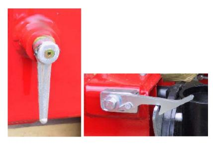
If the loader is equipped with swing-up stabilizer legs they must also be secured in position before driving off. Before the vehicle is started, disengage the PTO and turn off the pump.
