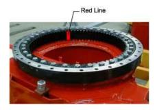
The external ring of the turntable must be oriented so that the filler plug next to the type plate turns towards the planetary gear. There is a hardened overlap next to the filler plug (ball groove).
