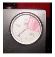
The load indicator dial shows the load moment pressure. When the load moment increases, the indicator approaches the red Danger Overload zone. When the indicator reaches the red zone, the loader is 100% loaded and the load on the loader must not be increased.
