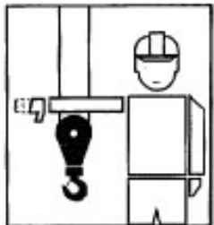
LOWER BOOM - RAISE LOAD Arm extended, thumb pointing down, flex fingers in and out until desired movement is completed.
