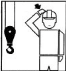
USE MAIN HOIST - Tap fist on head; then use regular signals.
