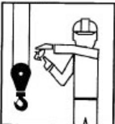
MOVE SLOWLY - One hand gives any motion signal; place other hand motionless in front of that hand. (Hoist slowly shown.)
