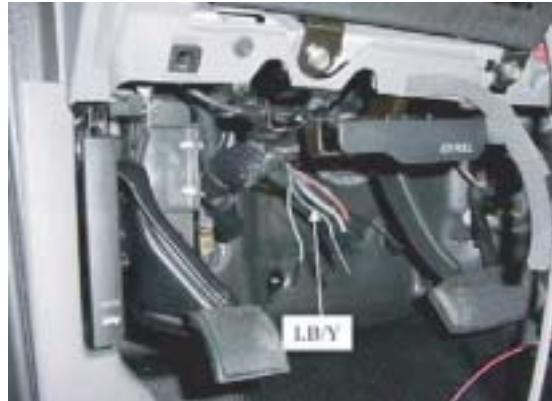
The PTO switch has a lt. blue / yellow wire that hooks up directly to the Ford-supplied circuit 322 (lt. blue / yellow).
