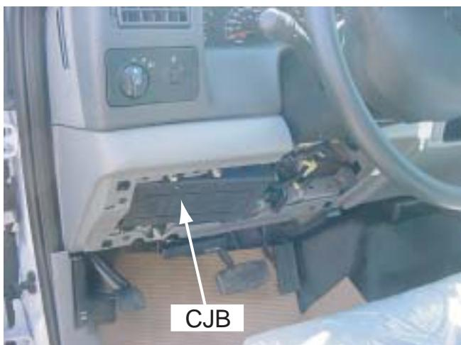
1. The Control Junction Box (CJB) is located behind the modesty panel below the steering wheel. Access to the engine kill and engine start wires are behind the CJB. Remove four bolts anchoring the CJB for access.
