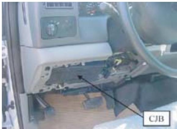
The CJB is located behind the modesty panel below the steering wheel. Access to the engine kill and engine start wires are behind the CJB. Remove the four bolts holding the CJB for access.
