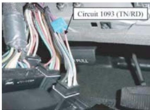
For engine start, splice into circuit 1093 (tan / red) in the location shown.
