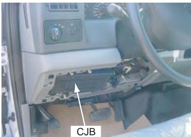
1. The Control Junction Box (CJB) is located behind the modesty panel below the steering wheel. Access to the engine kill and engine start wires are behind the CJB. Remove four bolts anchoring the CJB for access.
