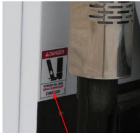
70392864 Warning-Stabilizer Stand Clear Decal shown on front sidepack (Typ 2)
