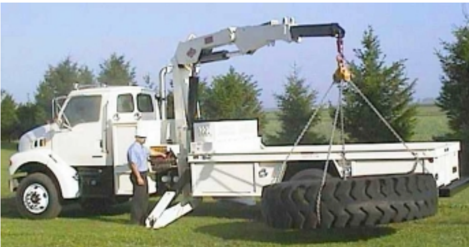
LIFT MADE IN HORIZONTAL POSITION
