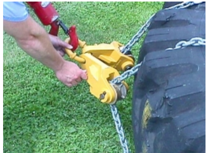
SECURING THE LOAD USING THE LOCK PIN
