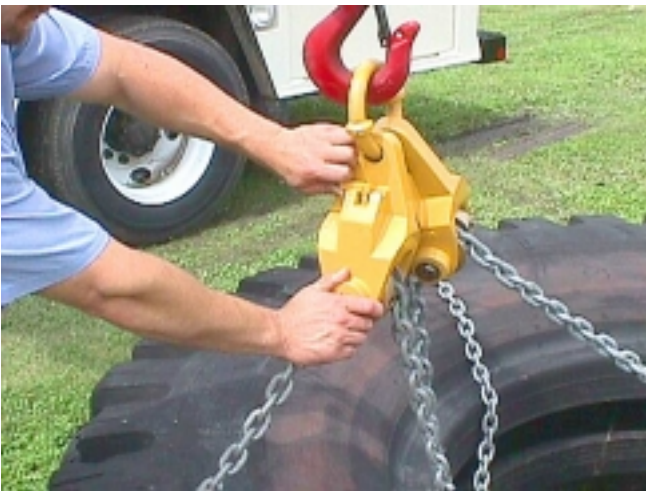
SECURING THE LOAD USING THE LOCK PIN
