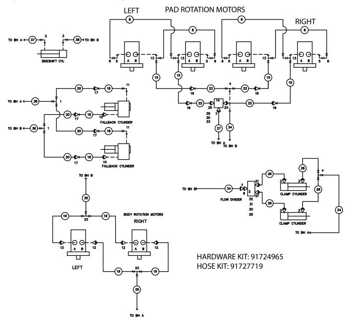
DWG 99906434 PROVIDES A BETTER REPRESENTATION OF THE OVERALL HYDRAULIC SYSTEM FOR A TH25 / TH36 SHORT ARM. VIEWED FROM THE LOADER SIDE OF TIREHAND.
