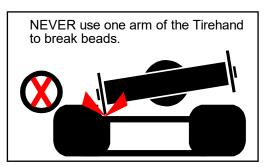
A bead breaker must be used to separate the tire from the rim. It is acceptable to use the Tirehand for holding the sidewall and flange away from the bead while o-rings and locking rings are being installed.
