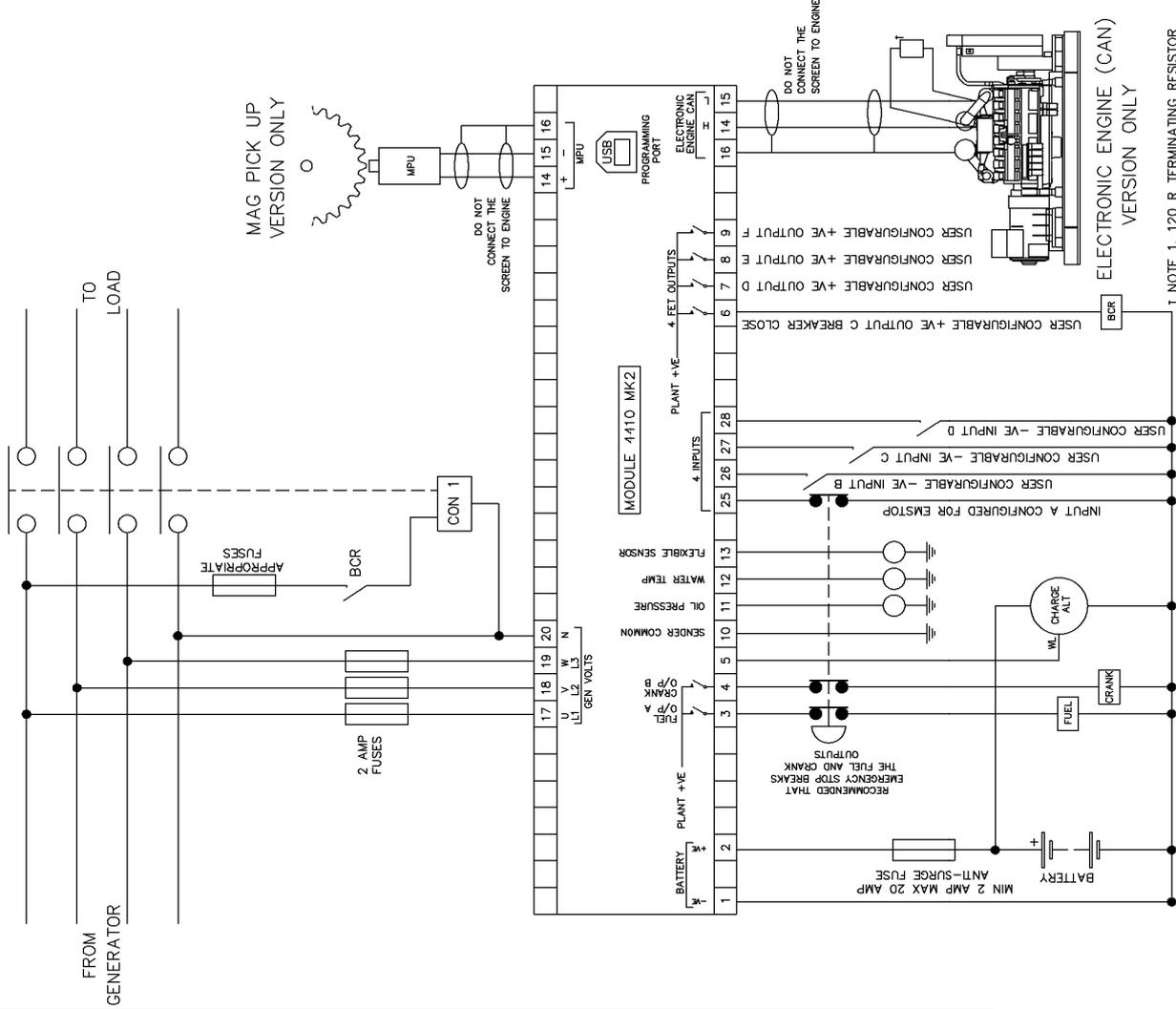
NOTE 1. 120 R TERMINATING RESISTOR MAY BE REQUIRED EXTERNALLY. SEE ENGINE MANUFACTURERS LITERATURE
