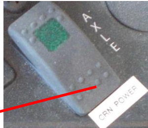
Crane Mode Switch
