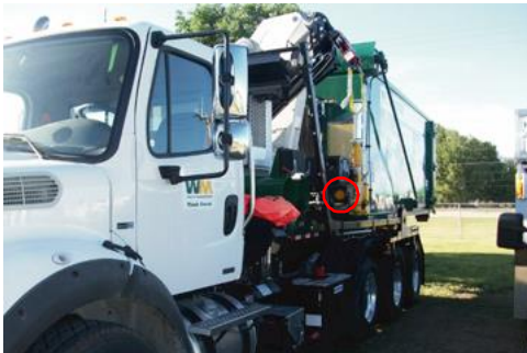
Reflective light which indicates when crane or stabilizers are not stowed.
