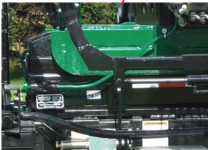
Front of roll-off container is secured in hooks on hoist.
