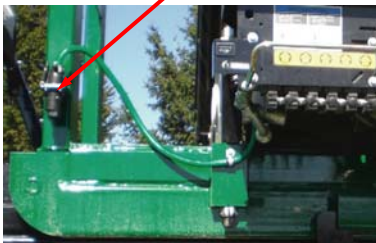
Stored position for green electrical cable
