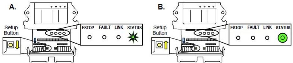
**NOTE:** If left idle in Setup Mode for over 30 seconds, the receiver will time out. The (Link) light and (Status) light will flash RED rapidly. To return to Setup Mode, repeat step 4.
