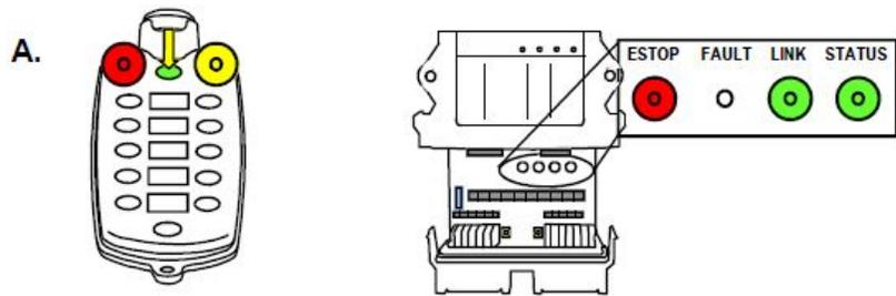
Once the ID Code has been downloaded, the RED (Battery) light and the YELLOW (Active) light on the transmitter will go out. The (Link) light on the receiver will change from GREEN to RED.
