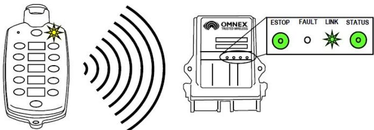
**NOTE:** The transmitter will shut itself off (and the receiver will then shut off all outputs) after 1 hour of inactivity as a battery saving feature. Momentarily operating any button on the transmitter, including the [Power] button will restart the 1 hour timer.
