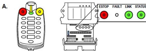
Once the ID Code has been downloaded, the RED (Battery) light and the YELLOW (Active) light on the transmitter will go out. The (Link) light on the receiver will change from GREEN to RED.
