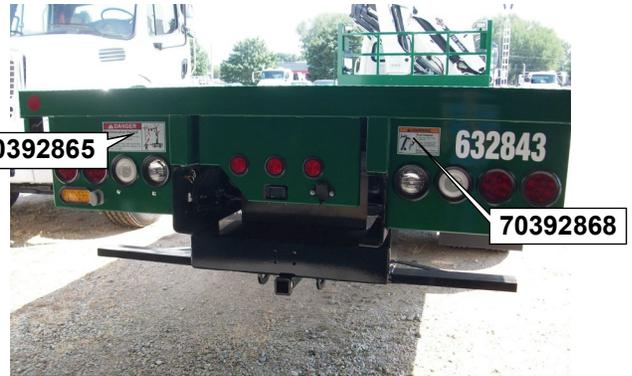
**NOTE:** The decal placement is typical on a flatbed CDV and a siderail CDV, except the rail height on a flatbed prohibits placement of the 70392865 and 70392868 on all 4 sides of the vehicle. Place 70392865 and 70392868 on the front and rear bumpers, and place 70396748 at the front and back corners of the flatbed sides. Place 70396918 crane safety decals (part of 95720380 crane kit) on the flatbed frame nearest the cab, next to the crane.
