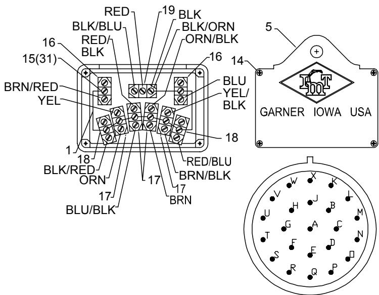
**Handle Assembly, Tethered Remote Kit (51713182)** (see "Handle Assembly, Tethered Remote (51713182)" on page 65)
