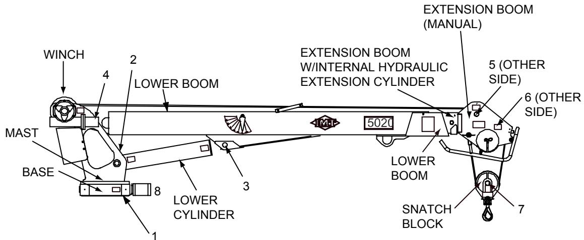
NOTE: Assemblies and part number locations are identified by name; grease zerk locations are identified by number.
