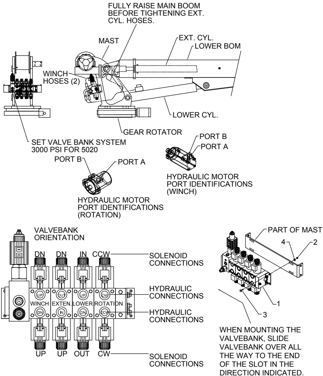
**Hydraulic Kit, Tethered Remote (91715636)** (see "Hydraulic Kit, Tethered Remote (91715636) & Radio Remote (91715571)" on page 47)
