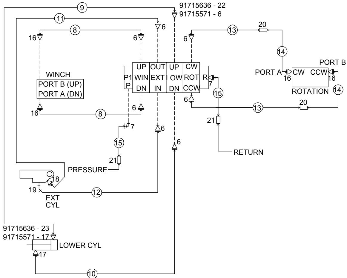
**Hydraulic Kit, Tethered Remote (91715636)** (see "Hydraulic Kit, Tethered Remote (91715636) & Radio Remote (91715571)" on page 47)
