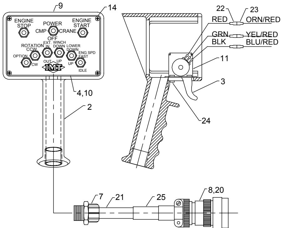
**Handle Assembly, Tethered Remote Kit (51713182)** (see "Handle Assembly, Tethered Remote (51713182)" on page 65)
