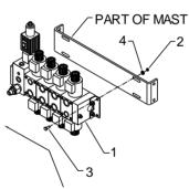
WHEN MOUNTING THE VALVEBANK, SLIDE VALVEBANK OVER ALL THE WAY TO THE END OF THE SLOT IN THE DIRECTION INDICATED.
