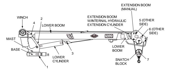
NOTE: Assemblies and part number locations are identified by name; grease zerks are identified by number.
