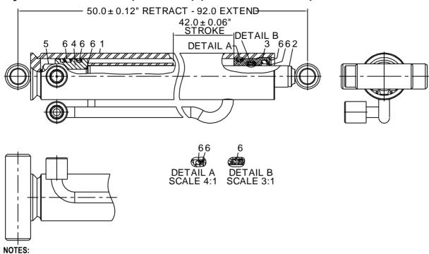
1 TO REDUCE DOWNTIME, REPLACE ALL COMPONENTS OF THE SEAL KIT WHENEVER THE CYLINDER IS DISASSEMBLED.
