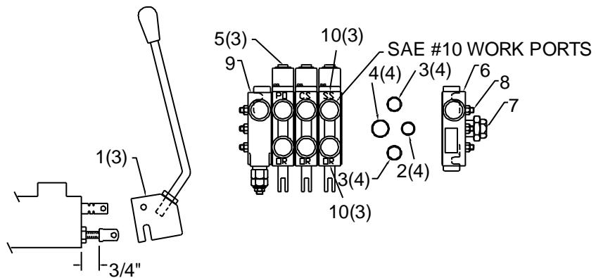
FOR OUTRIGGER VALVE BANK LEVER, PIVOT BOLT MUST BE HELD OUT 3/4" SO HANDLE TIPS IN AS SHOWN.
