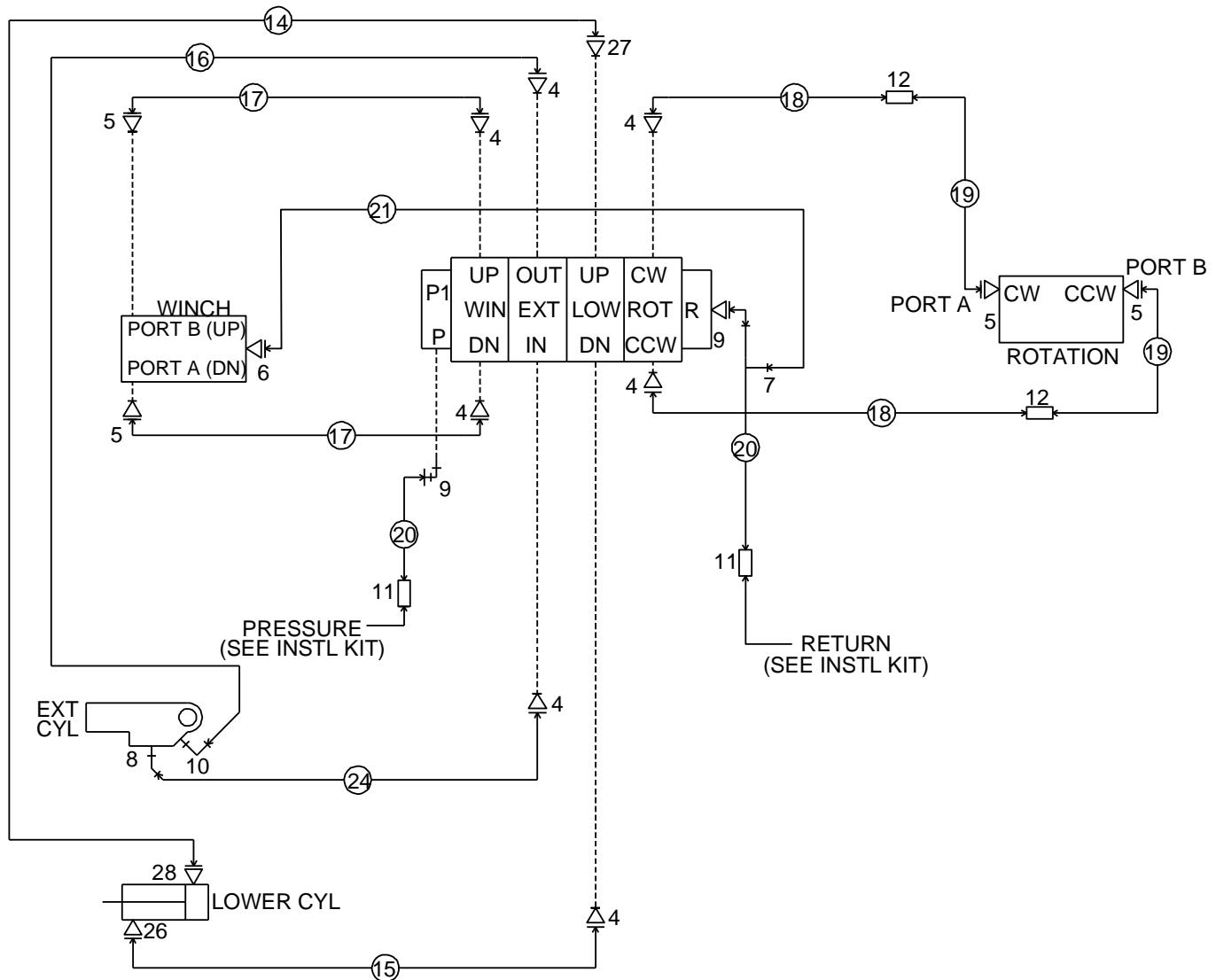
**Hydraulic Kit - Tethered Remote (91715637)** (see "Hydraulic Kit, Tethered Remote (91715637)" on page 62)
