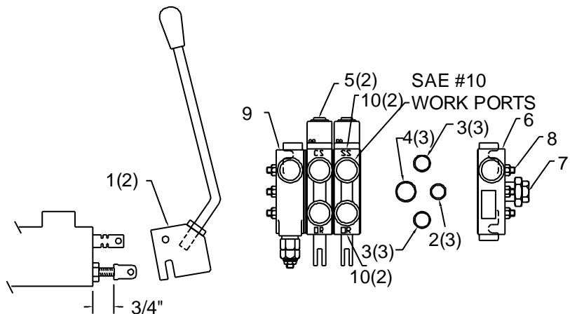
FOR OUTRIGGER VALVE BANK LEVER PIVOT BOLT MUST BE HELD OUT 3/4" SO HANDLE TIPS IN AS SHOWN.
