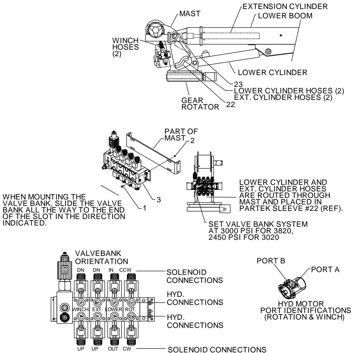
**Hydraulic Kit - Tethered Remote (91715637)** (see "Hydraulic Kit, Tethered Remote (91715637)" on page 62)
