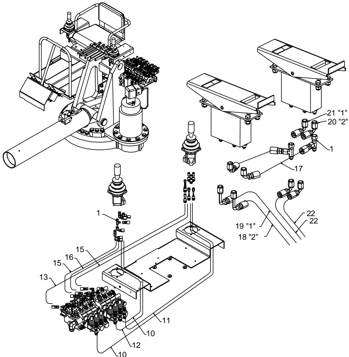
**Mast Assembly, Standard Controls (99903515)** (see "Hydraulics, Standard Controls (99903515)" on page 87))
