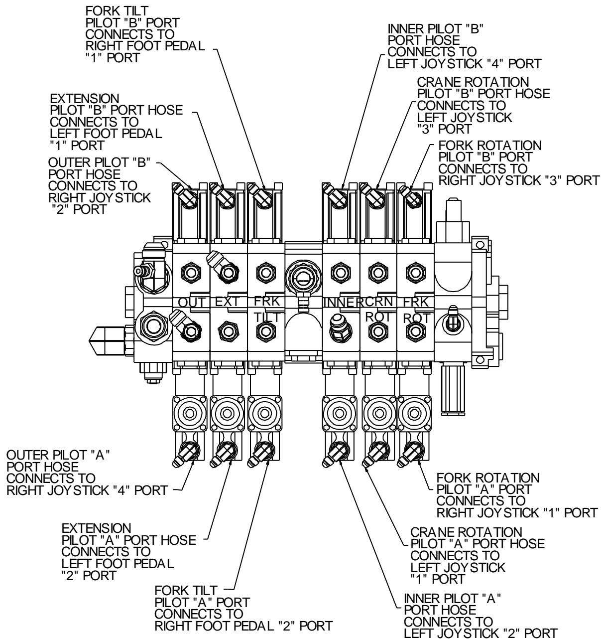
**Mast Assembly, Standard Controls (99903515)** (see "Hydraulics, Standard Controls (99903515)" on page 87))
