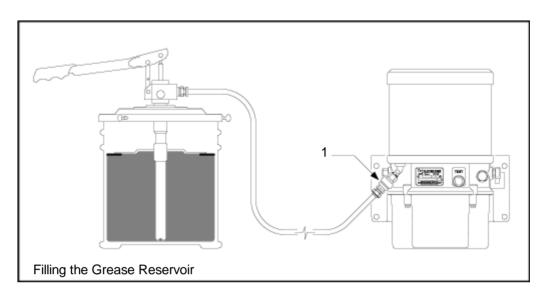
When the lubricant in the reservoir has fallen to the minimum level it must be refilled. Generally a filler pump is used for this purpose. The procedure is as follows:
