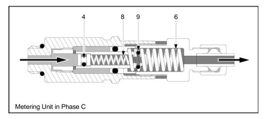
During the next lubrication cycle, the same happens as in phase A. Chamber (8) (Phase C), however, is now filled with grease. As plunger (4) moves right under influence of the grease pressure, the grease in chamber (8) is pressed, via chamber (6) and the secondary grease line, to the grease point.
