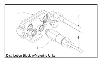
There are 11 metering unit types (1) available for the single line system, each with a differing metered lubricant quantity. By careful selection of the type of metering unit each lubrication point can be provided with the right quantity of lubricant.
