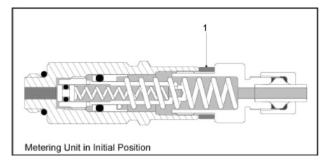
The figure above shows a new metering unit which has not yet been filled with grease. Item (1) in this figure is the spacer, which determines the delivery of the metering unit.
