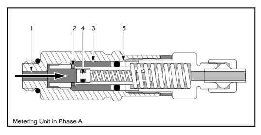
The pump presses the grease into grease channel (1). The grease pushes plunger (4) past channel (2). The grease now fills chamber (3) and pushes plunger (5) to the right. The stroke length of plunger (5) will determine the amount of grease that will be pressed through the secondary grease line to the grease point. This stroke length - hence the capacity of chamber (3) – is determined by the number and thickness of the spacers.
