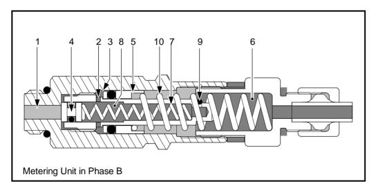
When the pump stops and as the grease pressure drops, spring (7) will push plunger (4) back to the left, closing off channel (1). O-ring (9) prevents grease from being sucked back from chamber (6). Plunger (5) is pushed back by spring (10) and presses the grease in chamber (3), via channel (2), to chamber (8).
