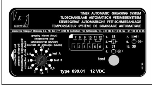
The greasing system is controlled by an electronic timer. The timer produces, at set time intervals impulses lasting 3 minutes. These impulses energize the solenoid value in the air supply to start the lubrication cycle. With an electrically operated pump the impulses start the pump. The interval between successive lubrication cycles is adjusted on the electronic timer.
