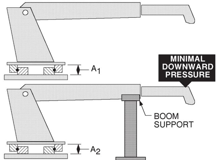
**COMPARISON CHART - MODEL TO MEASURED TILT DIMENSION**
