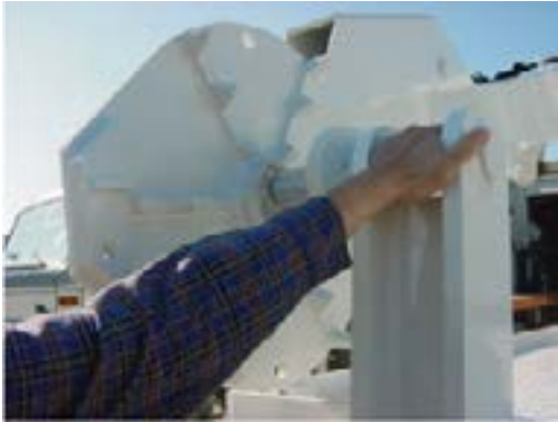
Example of stow mechanism pin being positioned into TireHand pad - street side.
