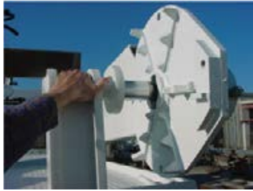
Example of stow mechanism pin being positioned into TireHand pad - curb side.
