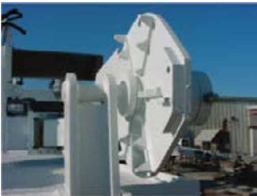
Full engagement of stow mechanism pin in TireHand pad.
