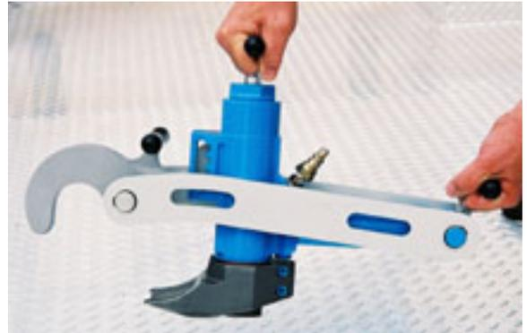
*Bead breaker with pin in lowest position.*
