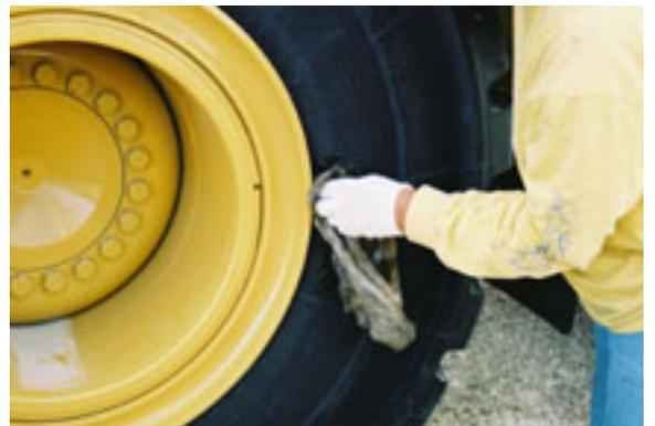
*Lubricate with rubber lubricant.*
