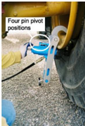
*The IMT Bead Breaker 1000 has four jaw pivot positions.*
