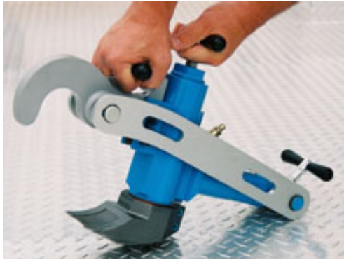
Bead breaker with pin in highest position.
