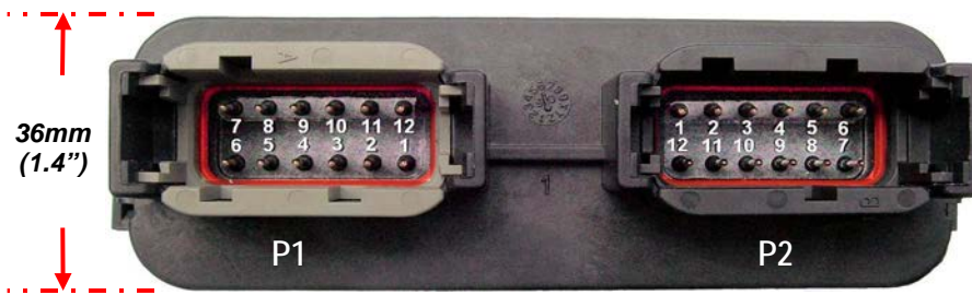
Figure 9: Receiver P1 and P2 Pinout
