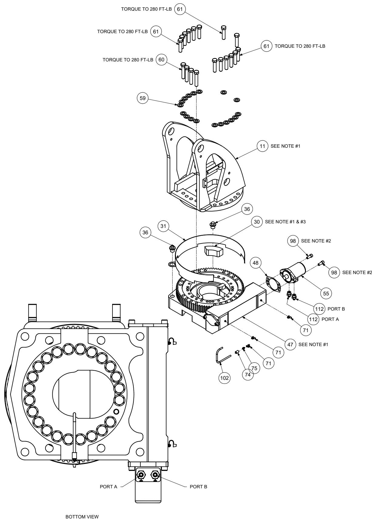
**BASE & MAST ASSEMBLY, TEST STAND PARTS LIST (99904922)**
