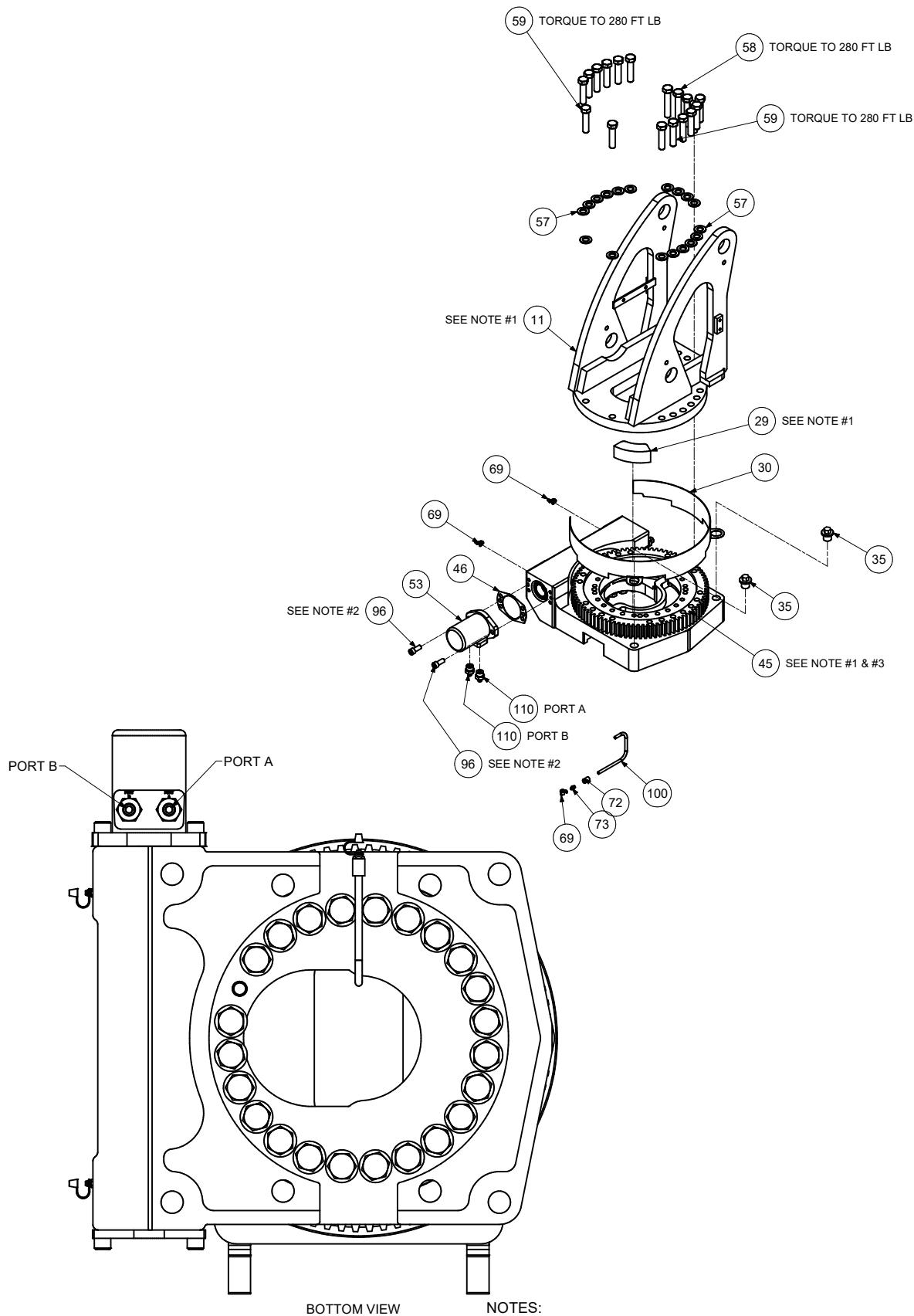
**99904925, BASE AND MAST ASSEMBLY, TEST STAND**
