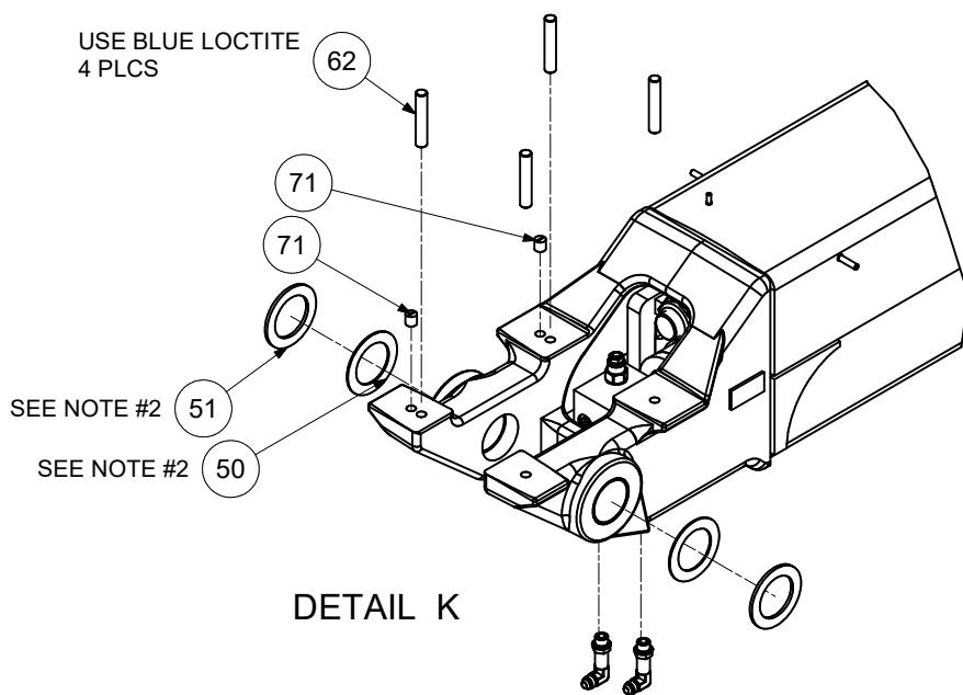
**CRANE & WINCH ASSEMBLY PARTS LIST (99904922)**
