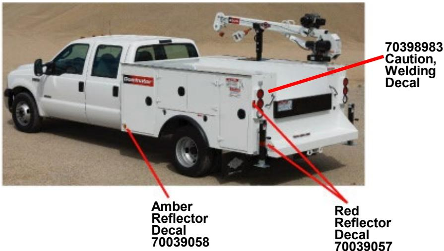
Four red reflector decals, 70039057, are located on each side and outer edge of the tailgate as shown.
