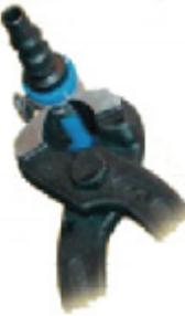
**NOTE:** Stepless ear clamps can only be used once. When removed, they must be discarded and replaced with new clamps.
