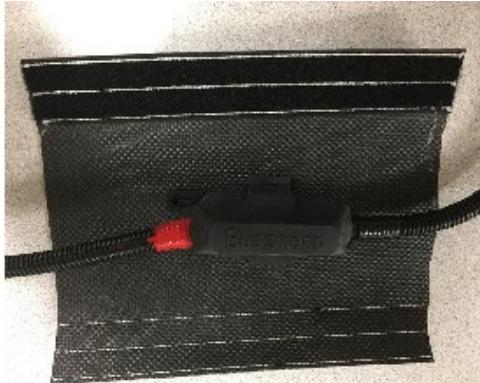
*Step 1: Place the protective sleeve under the fuse holder, centering the holder with the protective sleeve.*
