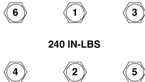
FIGURE E-2. CYLINDER HEAD TORQUE SEQUENCE
