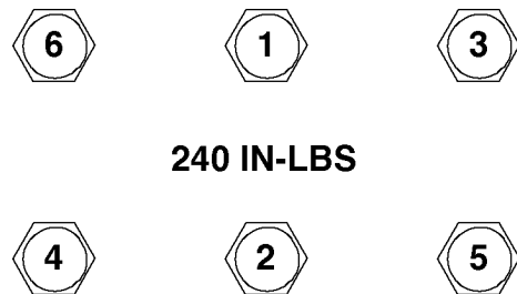
FIGURE E-2. CYLINDER HEAD TORQUE SEQUENCE
