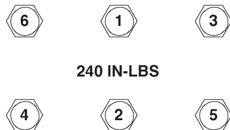
FIGURE E-2. CYLINDER HEAD TORQUE SEQUENCE
