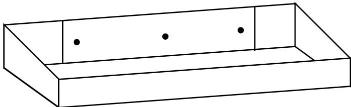
NOTE: Requires riveting. Rivets 72661226 included with assembly.
