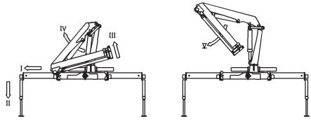
I. Extend stabilizer beams fully and check that the swivel locks are engaged.
