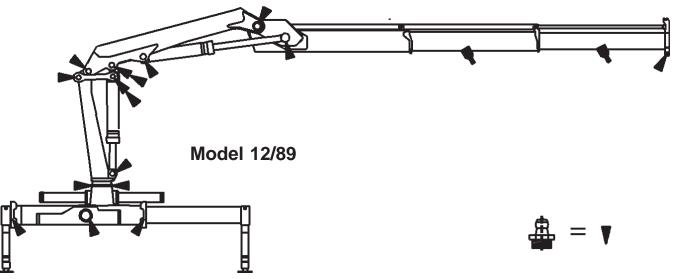
The rotation system should be activated and the loader swung from stop to stop several times within the whole rotation area at the same time as the bearings in the base are lubricated.
