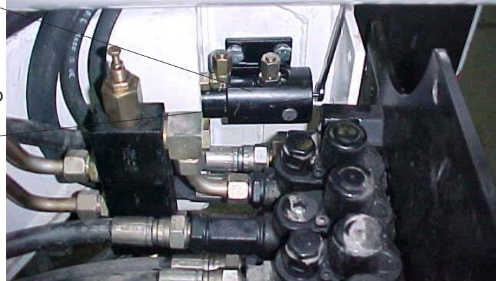
12. Once bracket is bolted in place, use 6 mm bolt to hold cylinder in place. This bolt tightens down flush to the bracket.
