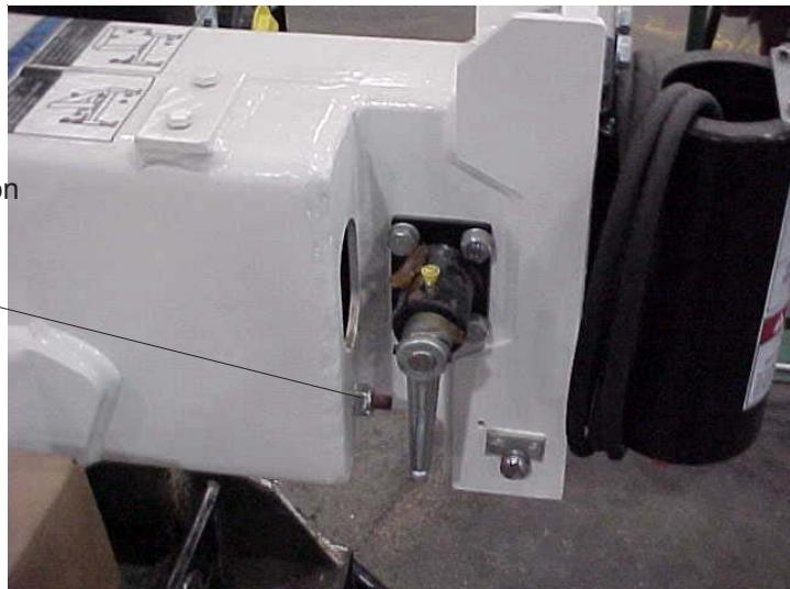
3. Remove the two bolts on the stabilizer stop.
