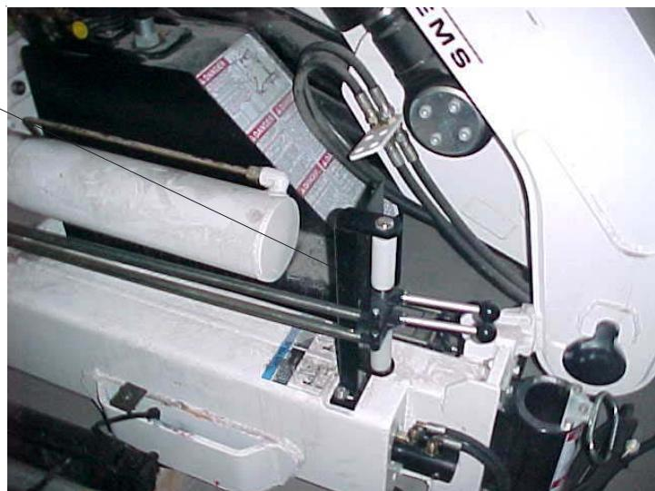
14. Bolt control rod bracket to the base on the curbside of the crane.
