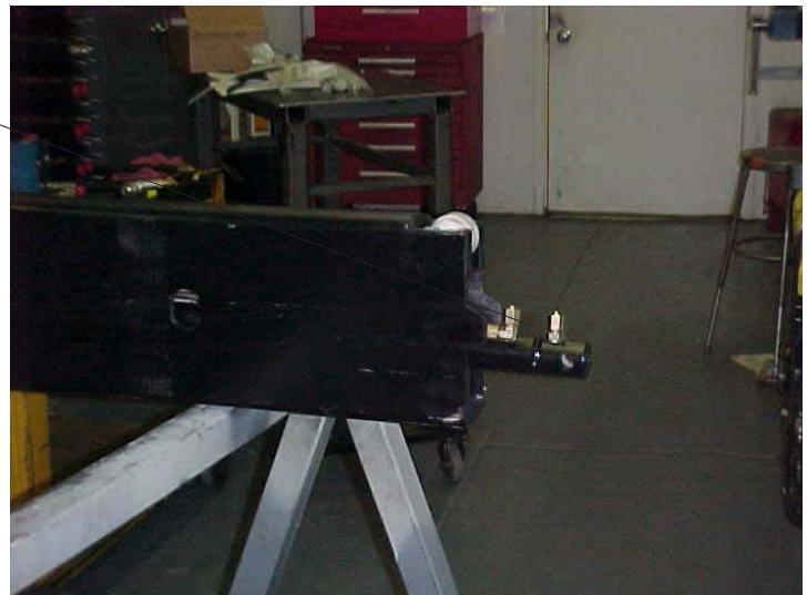
8. Install the stabilizer lock (removed in Step 1 from the crane curb-side) and wear pad on the inside of the crane.
