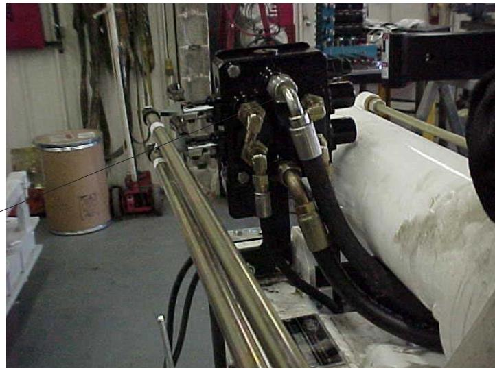
16. Port T1 is located on the valvebank bottom port next to the base. Remove the plug and screw in plug #61367. This must be installed to build up pressure so that the power stabilizers will function correctly. After installing plug, add fitting #25833. Connect hose #62848. The other end of the hose will connect to the two-section valvebank.
