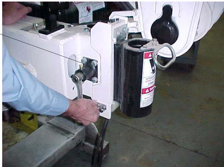
2. Remove nut on rod that comes through housing on both ends of crane base.
