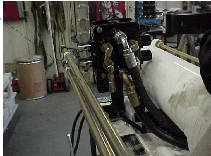
13. Bolt two-section valvebank onto base street side as shown.
