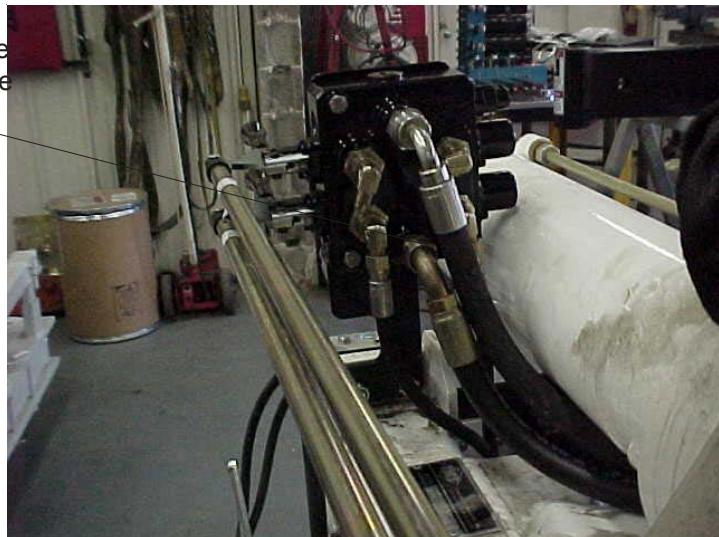
20. Run the 52" return hose from the two section valvebank to the tank on the front side of the crane as shown. Then, connect to the T on the tank.
