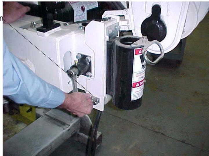
5. Remove this rod from the stabilizer. Set aside. This rod will not be used with the power-out kit.
