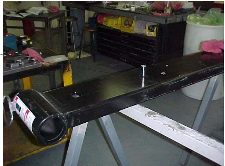
11. After sliding stabilizer back into the crane base, slide bracket on the end of the cylinder as shown. Pin bracket to cylinder, then bolt in place (4 bolts) to the crane base.
